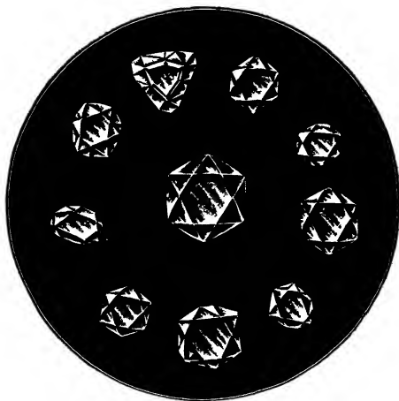
FIG. 125.—Ten Diamonds exhibiting Natural Faces, mounted for the Lantern Polariscope, to show Polarisation Colours due to Internal Strain
